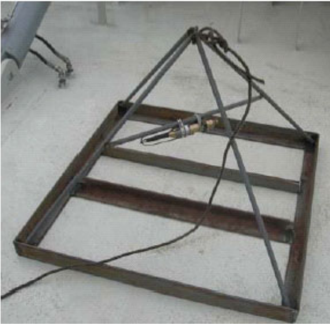
Fig. 5 Hydrophone attached to an example of a seabed cage
