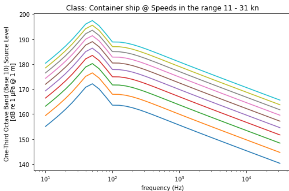
Figure 13. Noise spectra of various speeds of the ship class Container Ship. From top: 31 kn down to 11 kn in increments of two knots. The ship length in this example is 200 m. The one-third octave bands are calculated with base 10 (decidecade) according to the J-E model.
